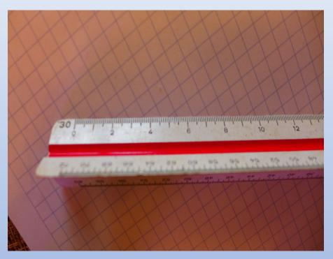
There are different marks (sides) on an engineer's scale The sides are 10, 20, 30, 40, 50, and 60 scales
